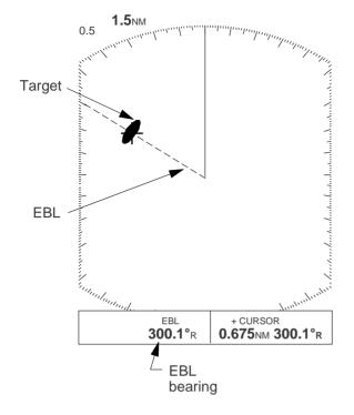
**To erase the EBL,** press and hold down the [EBL] key for about three seconds.
